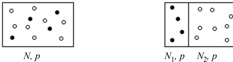
Figure 5.2. The two gases are mixed in the container to the left, but to the right they are separated by a wall so that the pressure is equal in the two parts.
